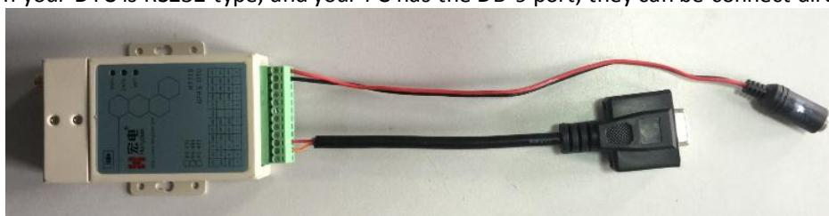
If your DTU is not RS232 type, you should prepare the convertor such as RS485-to-RS232 convertor;
